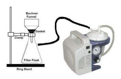
Remove the 250 mL beaker from the ice bath and transfer the mixture of alum crystals and liquid to the Buchner funnel QUICKLY. This is best accomplished by first swishing/swirling the contents of the beaker and then quickly dumping the contents into the Buchner funnel. Your lab instructor will demonstrate this technique.
