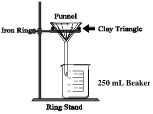
When cool enough to handle, pour the contents of the 250 mL reaction beaker into the gravity filtration apparatus assembled above. Use a glass stirring rod (right) to guide the liquid into the funnel. Don't overfill the funnel.
