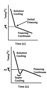
We could assume that the freezing point of the solvent in this case (pure water) should be  $0^{\circ}$ C. However, because we won't be calibrating the temperature probe, we cannot make this assumption. Instead, we'll measure the freezing point temperature of the pure water and use that value for  $T_{solvent}$ . Since we'll use the same temperature probe for all measurements (solvent and solutions), the error in each will subtract out as we calculate  $\Delta T$ .
